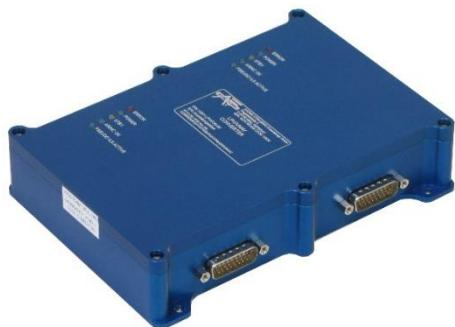
In ILS mode, the EFIS system expects ARINC429 localizer deviation, glideslope deviation and ILS energize information. If a LPV/VNAV approach is active, the LPV/VNAV-Converter switches the ARINC GPS output from the Garmin unit into the NAV input of the EFIS system. The LPV/VNAV-Converter extracts ARINC429 data and the DME compliant data from any SBAS capable FMS/GPS datastream and fits additional labels into the generated modified datastream to the EFIS system.
